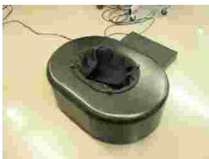
Fig. 2-1 : Three Dimensional Foot Scanner
