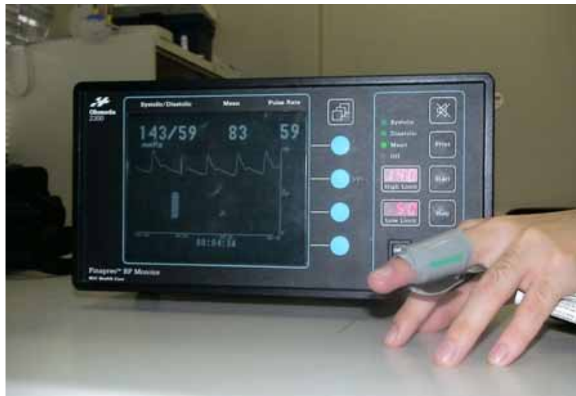
Fig.2 A Finapres noninvasive continuous blood pressure measurement.
